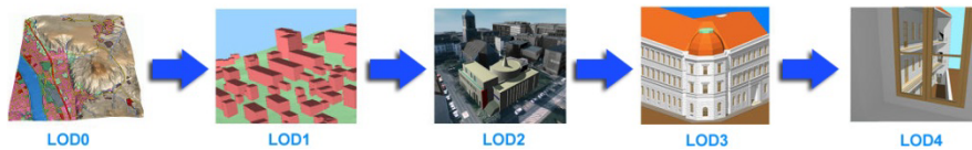
Figure 5 - A representation of how the Levels of Details change across the 5 LOD classes defined in CityGML specification (see Table 1 for detailed descriptions of LODs)
